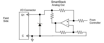
Specification for transient voltage suppressors (transorbs) used on output circuitry is 15V, 300W.
