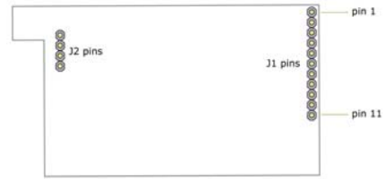
Figure 1.1. WCM802 / WCM900 OEM RF Module Pin Numbers (bottom view, pins protruding)
