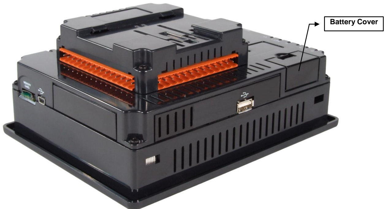
Figure 18.1 – Back Cover - Replacing the back-up battery
