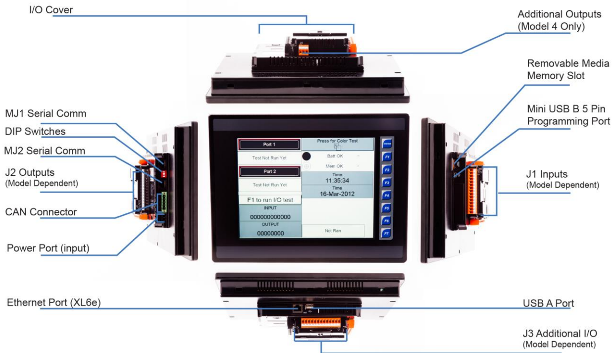
Figure 2.1 – Visual Overview of XL6(e) (above) and XL10e (below) OCS
