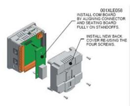
Figure 2 - Installing the COM Board in the XLE
