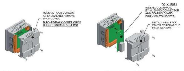
Figure 1 - Removing Back Cover of the XLE
