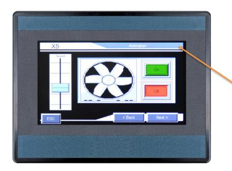
Press the far upper right corner to bring out the function keys and SYSTEM key in order to access the Main Menu.
