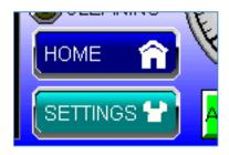
Figure 14.4- Typical Screen Jump Objects (X5)
