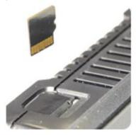
Figure 16.2 - Installing Removable Memory Card
