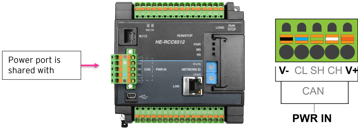
Figure 4.1 - Primary Power Port as Viewed Looking at the RCC6512
