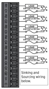
NOTE: Internal  $10k\Omega$  resistors between: V+ and Q1; V+ and Q2
