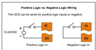
Digital inputs may be wired in either a Positive Logic or Negative Logic fashion as shown. The setting in the Cscape Hardware Configuration for the Digital Inputs must match the wiring used in order for the correct input states to be registered.
