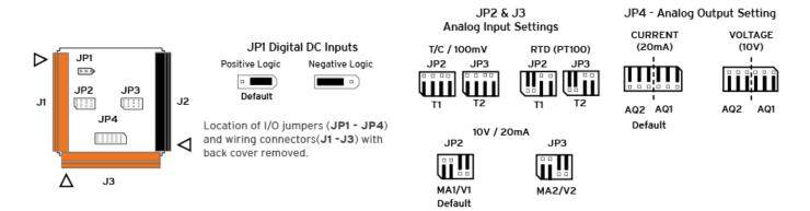
**NOTE:** The Cscape Module Configuration must match the selected I/O (JP) jumper settings. Path: Controller  $\rightarrow$  Hardware Configuration  $\rightarrow$  Local I/O  $\rightarrow$  Module Setup  $\rightarrow$  Analog I/O
