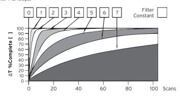
Analog filtering module response to a temperature change in the analog in. The illustration above demonstrates the effect of digital filtering on (set with Filter Constant).
