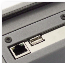
The RX371 is designed for harsh environment use, with its metal chassis, ruggedized heavy duty function keys and impact resistant touch screen. Snap-on I/O is provided by metal SmartStack® units or SmartStix® I/O.
