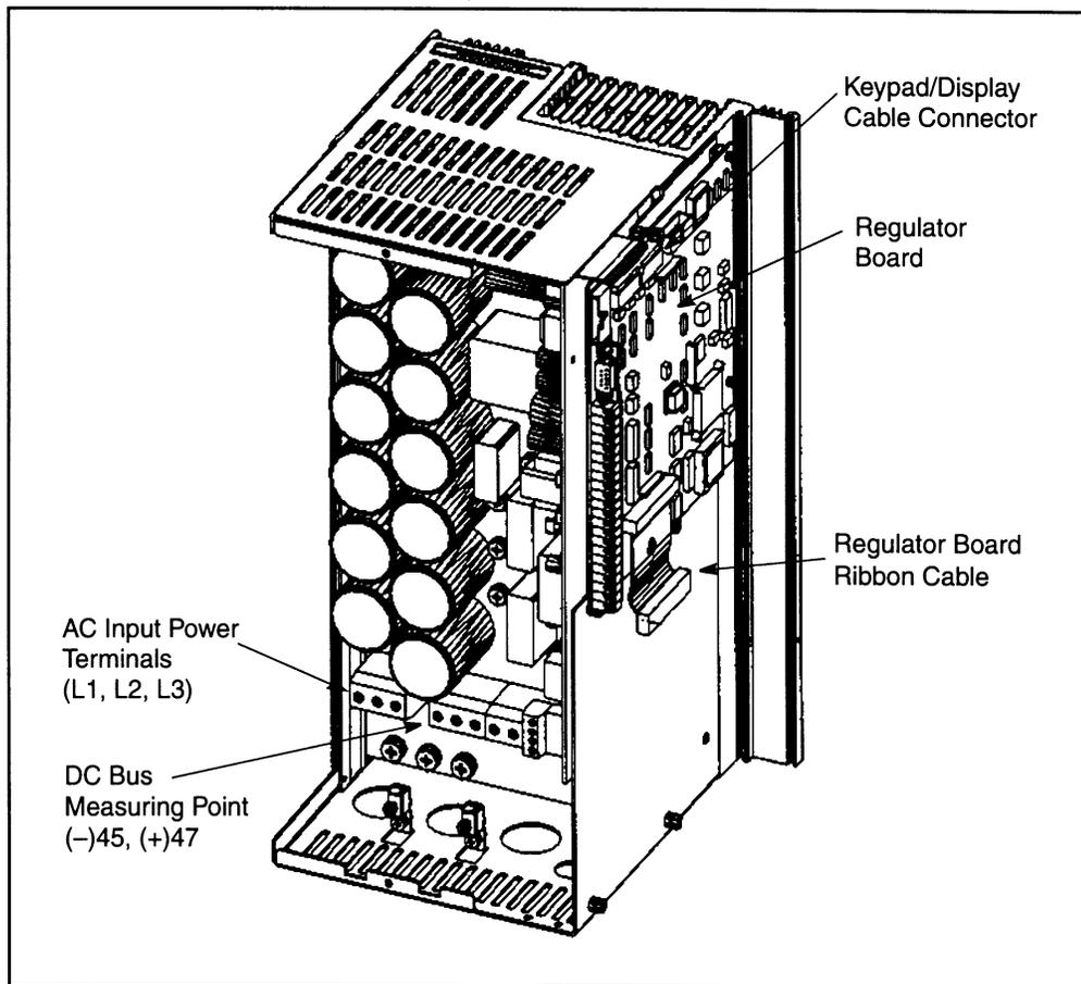
Figure 2.19 – 24 to 30 Amp Bookshelf Drive (cover and Front Panel Removed)
