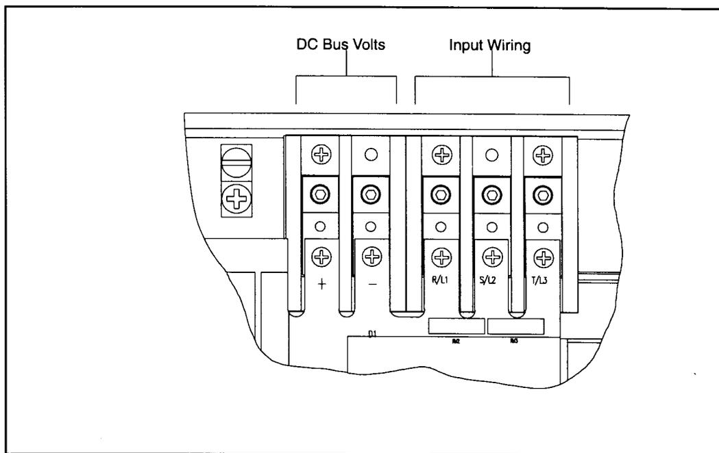
Figure 2.12 – DC Bus Voltage Terminals (25 to 60 HP @ 460V)
