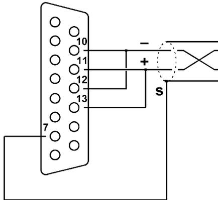
Figure 2.22 – FLN cable connection to DB15
