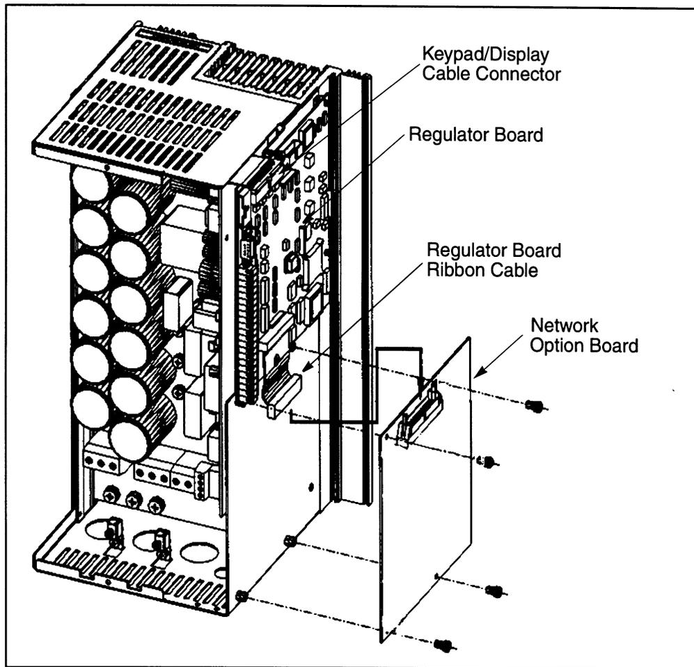
Figure 2.20 – Installing the Network Option Board in Bookshelf Drive
