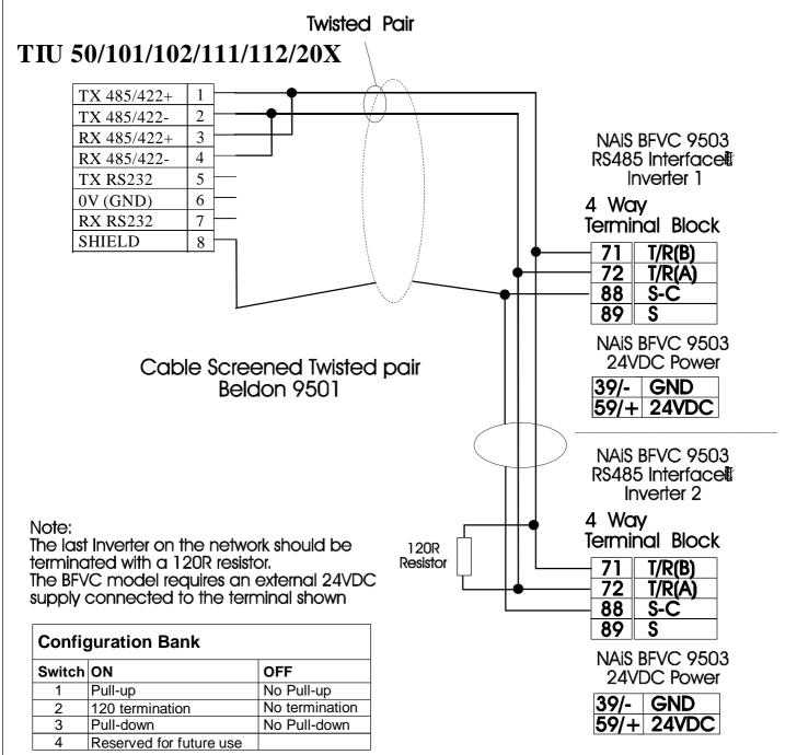
NOTE: Switch 1 and 3 must be used together.
