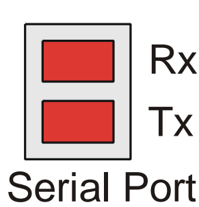
Figure 4.4 – Automation Equipment Port Receive & Transmit LEDs The LED's flash when the HE500TIU100/110 is communicating.
