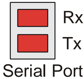
Figure 5.4 – Automation Equipment Port Receive & Transmit LEDs The LED's flash when the HE500TIU100/110 is communicating.
