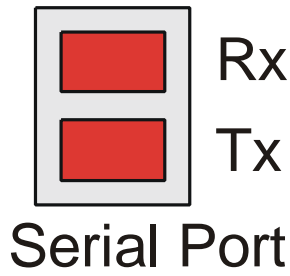
Figure 3.4 – Automation Equipment Port Receive & Transmit LEDs
