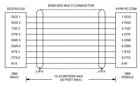
Figure 8- OCS to PC Wiring Diagram
