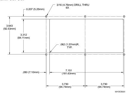
Figure 1 - Panel Cut-Out for the OCS100/110
