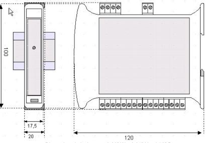
Dimensions in inches are 0.69" W x 3.95" H x 4.72" D Note: Number of I/O terminal connections varies from model to model.
