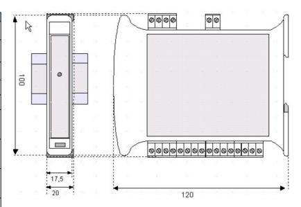
Dimensions are 0.69" W x 3.95" H x 4.72" D Note: Number of I/O terminal connections varies from model to model.
