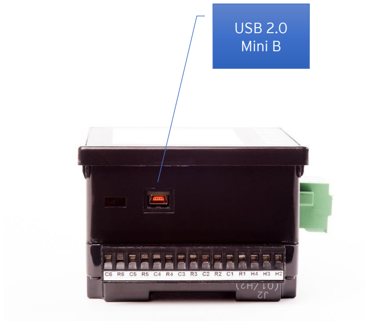
Figure 7.1 - USB Programming Connector
