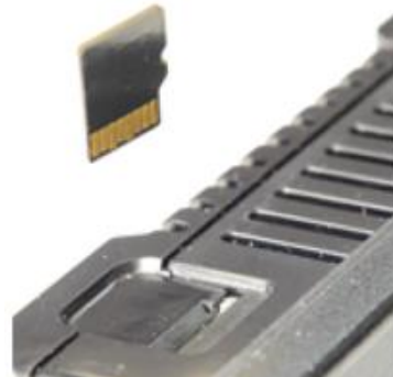
Installing Removable Memory Card
