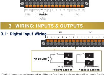
Digital inputs may be wired in either a Positive Logic or Negative Logic fashion as shown. The setting in the Cscape Hardware Configuration for the Digital Inputs must match the wiring used in order for the correct input states to be registered. The state of the inputs are reflected in registers %I1 - %I8. The Common connections are found on the top connector.
