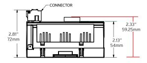
Clearance Requirements Top and Bottom: 1" or 25.4mm Sides: 0.5" or 12.7mm
