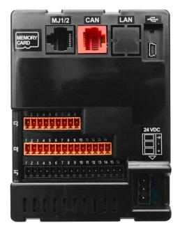
Figure 11.1 - CAN Connector (Red)
