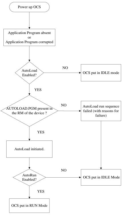
Figure 16.7 - Flow Chart for AutoLoad
