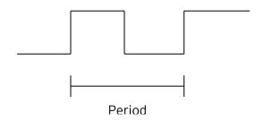
Figures 9.7 & 9.8 - PWM, two parameters, Duty Cycle & Frequency
