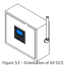
**NOTE:** For panel mounting–The orientation shown provides for optimum readability screen and ease of use of the keypad.
