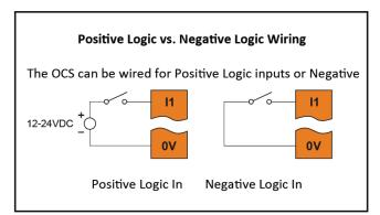
Figure 8.5 - Positive and Negative Inputs
