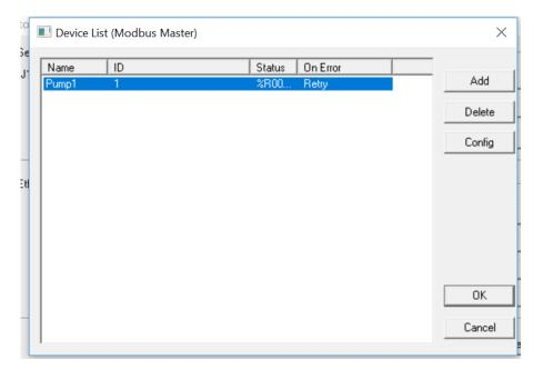
The Device List is reached from the Device button on the Protocol Config screen and provides a list of the configured devices on the Network. Devices must be created and exist in this list before corresponding Scan List entries can be created for this device. Typically, the number of entries is limited to **64 devices**.
