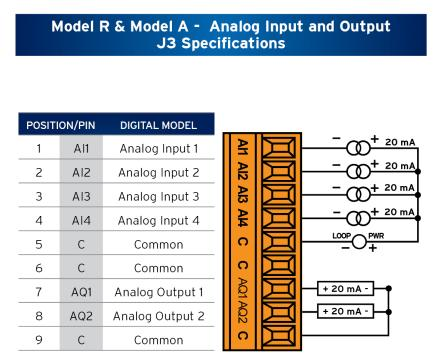
Figure 8.7 - Model R and A Analog In and Out
