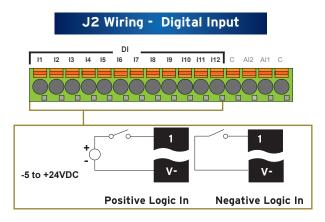
Digital inputs may be wired in either a Positive Logic or Negative Logic fashion as shown. The setting in the Cscape Hardware Configuration for the Digital Inputs must match the wiring used in order for the correct input states to be registered. The state of the inputs are reflected in registers %I1 through %I12. The Common connections are found on the top connector. Inputs 1-8 have programmable input voltage ranges and input frequency filters.
