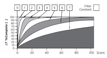
Digital filtering module response to a temperature change in the analog in. The illustration above demonstrates the effect of digital filtering on (set with Filter Constant).
