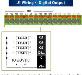
Digital outputs are Positive Logic. If an output is turned on, the voltage supplied at the QV+ terminal is applied to that output. When used as normal inputs, the state of the output may be controlled using the registers %Q1 -%Q10.
