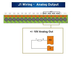
Each Analog Output may be specified for a range of -10VDC to +10VDC. The Analog Output registers %AQ1 - %AQ4 may be used to control the output by placing a value between - 32000 to +32000 into the register. This may be directly from a PID loop output, for example.
