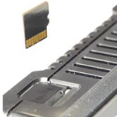
Figure 15.2 - Installing Removable Memory Card
