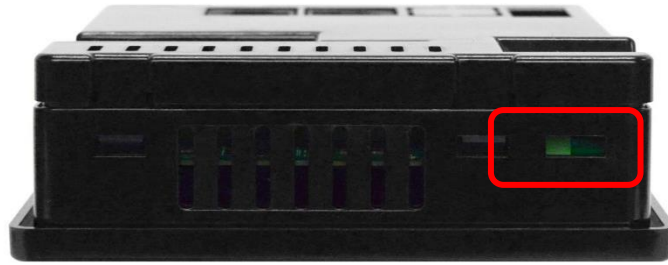
Figure 3.1 - X4 OCS with Mounting Clip Location
