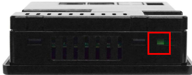
Figure 3.1 - X7 OCS with Mounting Clip Location
