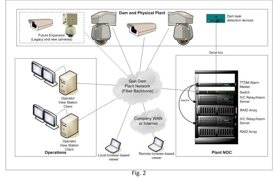
**Figure 2** illustrates a functional diagram of the video surveillance system we have described in this application note. A key reason IVC was chosen to provide the video system for this major upgrade project by ABB, is that, as a provider of quality industrial-grade video cameras and camera management software, IVC was wellpositioned to tailor a solution to exactly meet the needs of ABB and their customer. Our
