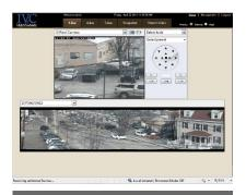
IVC's Tour Manager software allows the user to program a specific view and time intervals, allowing the camera to take a single picture or series of pictures at regular intervals. When strung together these form a time-lapse view of the construction process.
