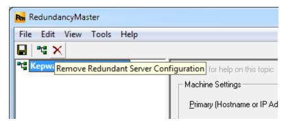
After a redundant server configuration has been removed, the redundant server will still be displayed in the OPC Server Browser window. To update the list of servers, click **Refresh**. To refresh the browser window, right-click on the machine name and then click **Refresh**. Afterwards, the redundant server that was removed should no longer be displayed.
