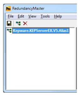
3. Once one redundant pair has been aliased, another redundant pair can be created. An alias can then be assigned to that pair (such as, *ServerProgID*.Alias2).
