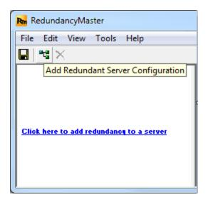
3. Next, locate and select the ProgID of the OPC server to which redundancy will be added. This OPC server may be on the local or remote machine.
