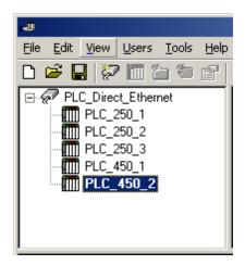
Each device appears under a single AutomationDirect ECOM channel. In this configuration, the driver must move from one device to the next as quickly as possible in order to gather information at an effective rate. As more devices are added or more information is requested from a single device, the overall update rate begins to suffer.
