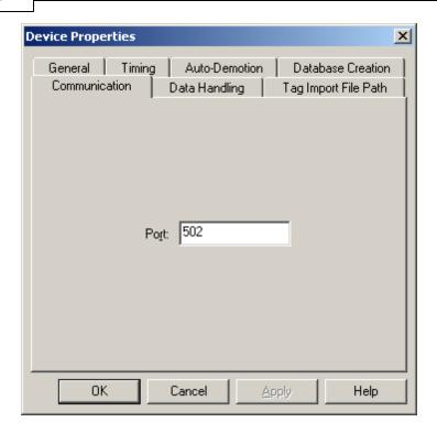
Note: The default communication protocol is Modbus TCP/IP.
