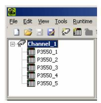
Each device appears under a single AutomationDirect Productivity 3000 Ethernet driver channel. In this configuration, the driver must move from one device to the next as quickly as possible in order to gather information at an effective rate. As more devices are added or more information is requested from a single device, the overall update rate begins to suffer.
