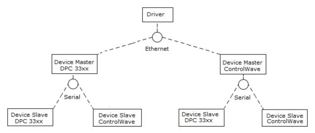
The Bristol BSAP IP Driver communicates to Master or Slave devices using Ethernet (UDP). Communications to Master devices are direct: the driver sends a request to the device and it responds. Communications to Slave devices are indirect: the driver sends a request through the Master device. In most configurations, Slave devices communicate over serial to the Master.
