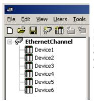
Each device appears under a single Cutler-Hammer ELC Ethernet channel. In this configuration, the driver must move from one device to the next as quickly as possible in order to gather information at an effective rate. As more devices are added or more information is requested from a single device, the overall update rate begins to suffer.
