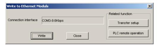
There must be a serial connection to the FX3U PLC because the configuration settings are written to the PLC via this serial link. Make sure that the communication parameters are correct by using the **Transfer setup** button above or by clicking **Online** | **Transfer setup** from the main menu.
