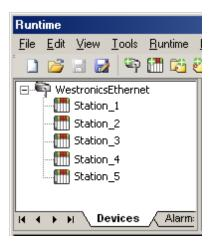
Each device appears under a single Thermo Westronics Ethernet channel. In this configuration, the driver must move from one device to the next as quickly as possible in order to gather information at an effective rate. As more devices are added or more information is requested from a single device, the overall update rate begins to suffer.
