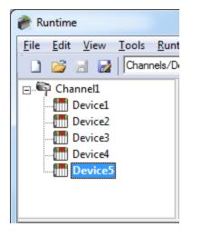
Each device appears under a single Torque Tool Ethernet channel. In this configuration, the driver must move from one device to the next as quickly as possible in order to gather information at an effective rate. As more devices are added or more information is requested from a single device, the overall update rate begins to suffer.
