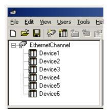
Each device appears under a single Yokogawa CX Ethernet Device channel. In this configuration, the driver must move from one device to the next as quickly as possible in order to gather information at an effective rate. As more devices are added or more information is requested from a single device, the overall update rate begins to suffer.
