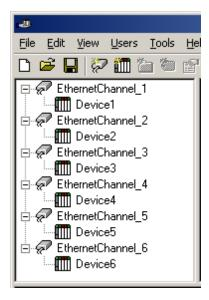
Each device has now been defined under its own channel. In this new configuration, a single path of execution is dedicated to the task of gathering data from each device. If the application has 16 or fewer devices, it can be optimized exactly how it is shown here.
