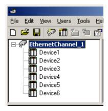
Each device appears under a single Yokogawa DX Ethernet Device channel. In this configuration, the driver must move from one device to the next as quickly as possible in order to gather information at an effective rate. As more devices are added or more information is requested from a single device, the overall update rate begins to suffer.
