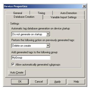
The **Automatic Tag Database Generation on device startup** selection is used to configure when OPC tags will be automatically generated. There are three possible selections. Descriptions are as follows:
