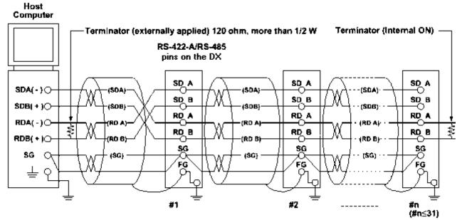
No terminators are inserted between #1 through #n-1 (internal OFF)
