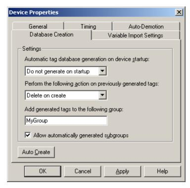
**Automatic tag database generation on device startup** is used to configure when OPC tags will be automatically generated. There are three possible selections:
