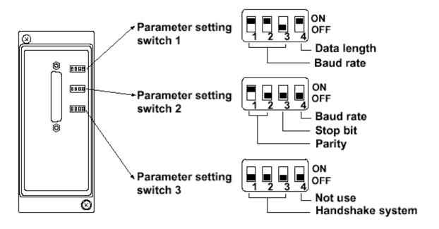
Baud Rate (No.1 to 3 of Setting Switch 1 and No.4 of Setting Switch 2) Baud Rate No.1 No.2 No.3 No.4 (Switch 2)
