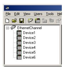
Each device appears under a single Yokogawa MX Ethernet Device channel. In this configuration, the driver must move from one device to the next as quickly as possible in order to gather information at an effective rate. As more devices are added or more information is requested from a single device, the overall update rate begins to suffer.
