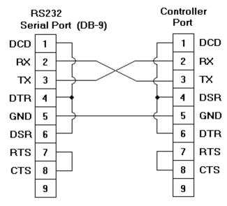
**Note:** The diagram above is a typical cable connection. For connection options, refer to the documentation that came with the device.
