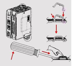
Rail mounting: DIN rail 35mm.
