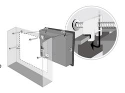
Minimum required clearances (along the overlay): Top / Bottom / Sides 15 mm Maximum panel thickness: 4.5 mm
