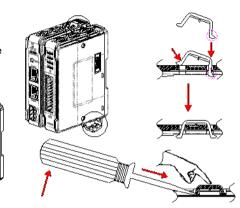
Rail mounting: DIN rail 35mm.
