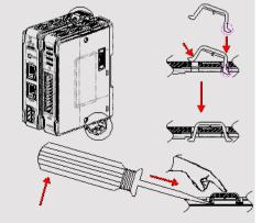
Rail mounting: DIN rail 35mm.
