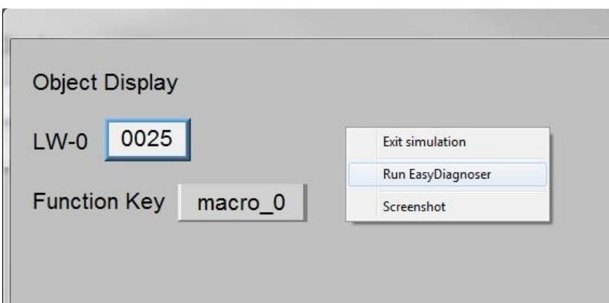
5. EasyDiagnoser will start and the Logger window at the bottom of EasyDiagnoser will indicate “Connection established with the target HMI.”
