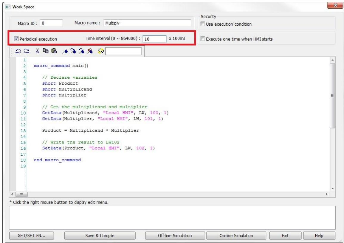
2. In the Macro Work Space, select “Execute one time when HMI starts” to run the macro once when the HMI is first turned on or rebooted.
