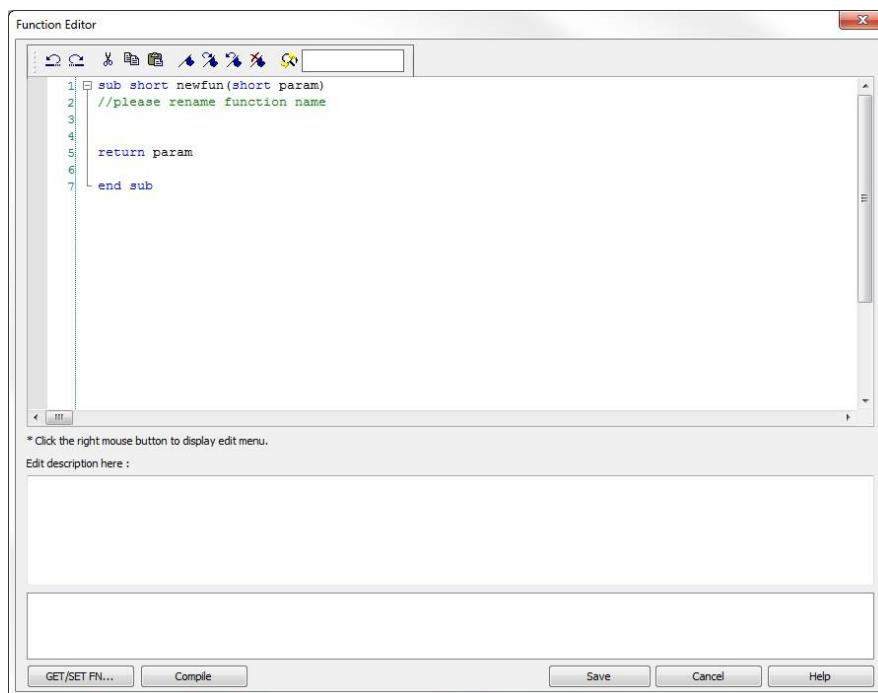
Edit the function according to the required format. You can use the description field at the bottom of the Function Editor to describe what the function does, how to use it, etc.
