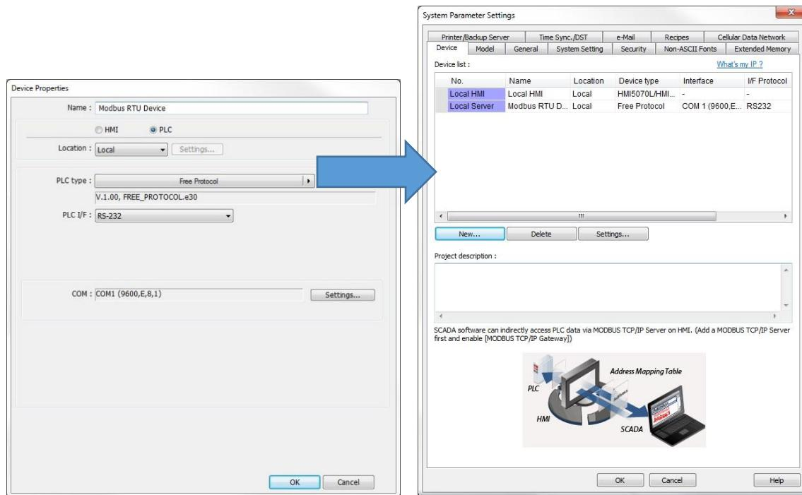
The above example uses RS-232 for the PLC I/F (PLC interface). If the interface of the Modbus device uses Ethernet (Modbus TCP/IP), select Ethernet for the PLC I/F with the correct IP address and port number in the Device Properties:
