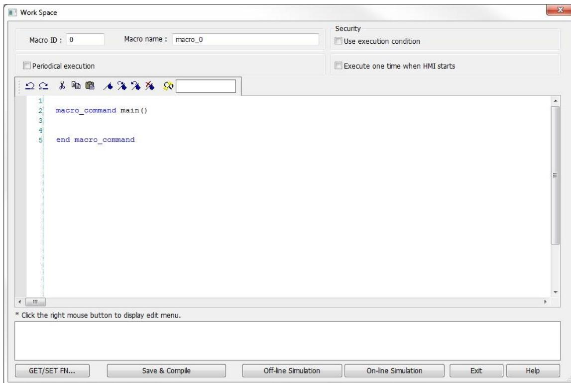
3. Design your macro. To use built-in functions like SetData() or GetData(), click the “GET/SET FN...” button to open the API dialog box. Select the function and set the appropriate parameters.
