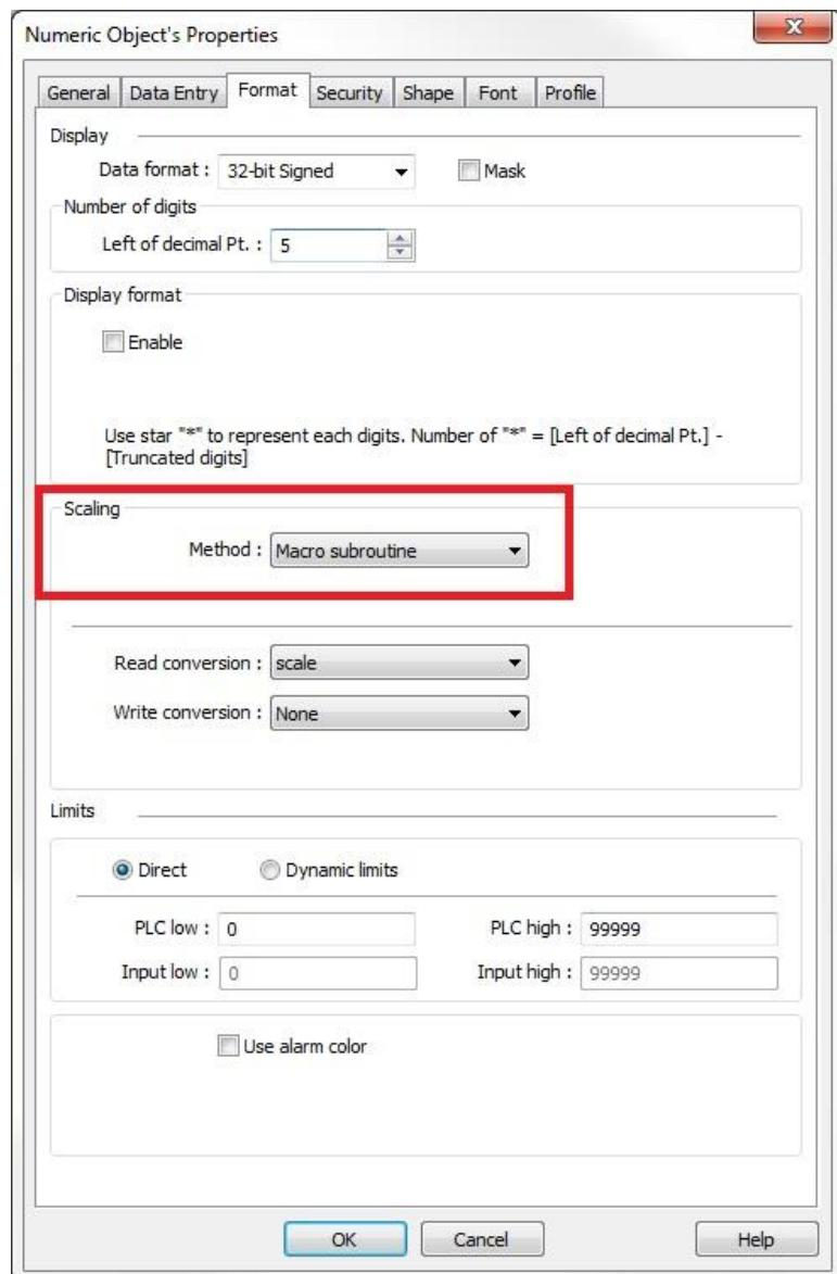
When “Allow input” is selected on the General tab, a macro function from the Macro Function Library can be assigned to the Read and Write actions of the Numeric object independently.
