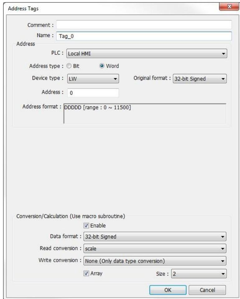
Enable the “Conversion/Calculation” option. A macro function from the Macro Function Library can be assigned to the Read and Write actions of the Address Tag independently. When the tag is assigned to an object, the macro function is applied to the read or write value that is displayed or written.
