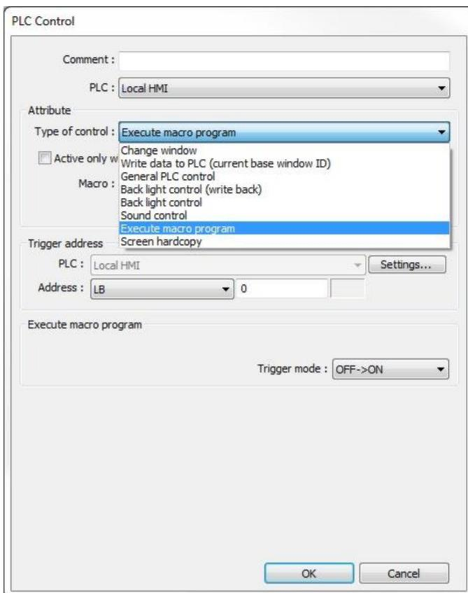
3. Select the macro you wish to execute under "Macro." Under "Trigger address," choose a bit and select a trigger condition to trigger the macro. In order to guarantee that the macro will run only once, consider latching the trigger bit and then resetting the trigger condition within the macro.
