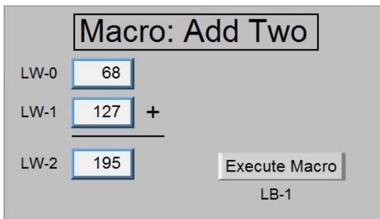
The operator enters a number in the Numeric object LW-0 and LW-1, then presses the “Execute Macro” button. This turns ON LB-1 and triggers the PLC Control object to execute the macro “AddTwo.” The macro adds the values in LW-0 and LW-1, writes the result to LW-2, and clears LB-1 so that the macro can be triggered again.
