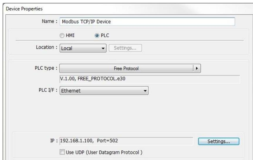
2. Suppose you want the HMI to read the data from 4x-1 and 4x-2 on the device. First, use the OUTPORT function to send out a read request to the device. The format of OUTPORT is:
