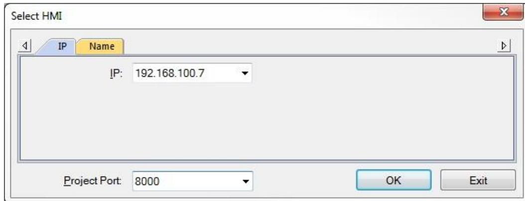
The Project Port number must match the Port no. in the EZwarePlus project's System Parameters > Model tab.
