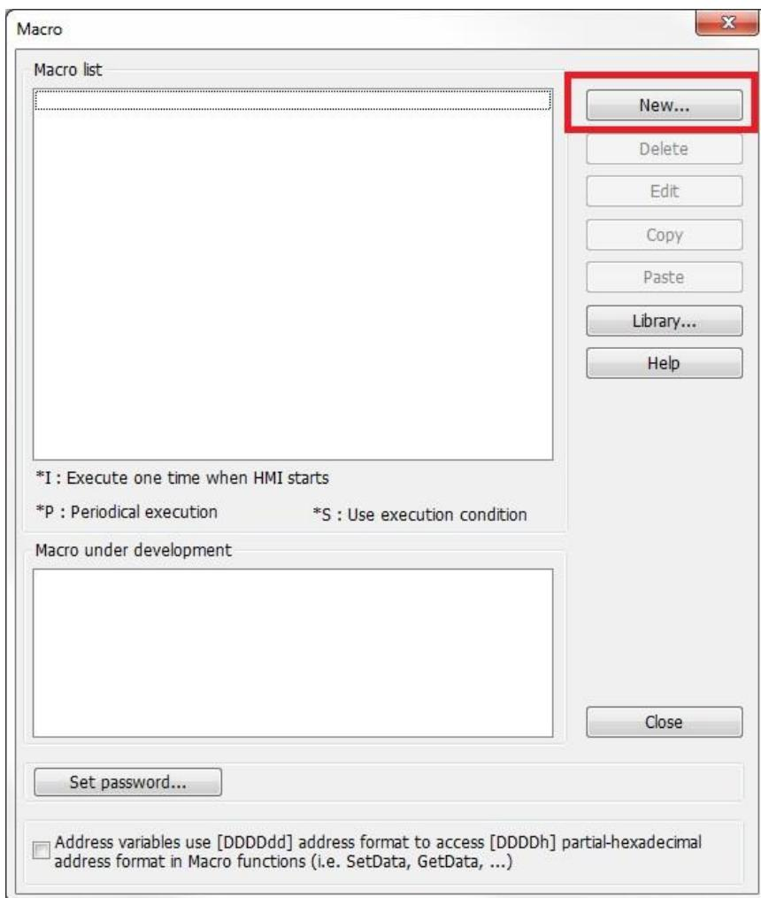
3. The Macro ID number is automatically assigned when the macro is created but can be changed to reorder the macros in the list. The programmer can give a name to the macro or simply use the default name (for example, macro\_0).
