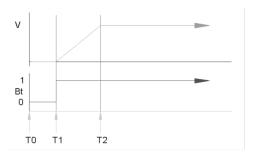
Closed loop speed control based on position over time, not frequency. This means that from the initial command to begin motion, the controller keeps track of what the actual position should be.
