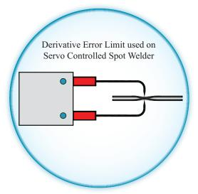
Jaw stops immediately upon making contact with metal for minimal product deflection and maximum balance to each side.
