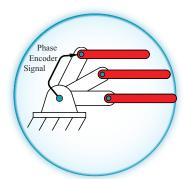
Enables applications such as product tracking where moves must be applied over a target in motion, automatically stabilizes pan & tilt applications, or allows arm end effectors to remain parallel to base while the mid arm section moves.
