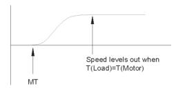
Open loop directional control of power to the motor windings. In this mode the motor has knowledge of encoder position but does not use it for motion. The motor will increase speed until its commanded torque equalizes with load torque. If load torque decreases, shaft speed will increase. If load torque increases, shaft speed will decrease. In a static condition, force applied will be proportional to commanded torque.
