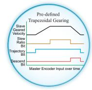
Now includes separate Ascend, Slew and Descend pre-defined distances that may be defined off of either master or slave encoder values for enhancing applications such as high speed winders.
