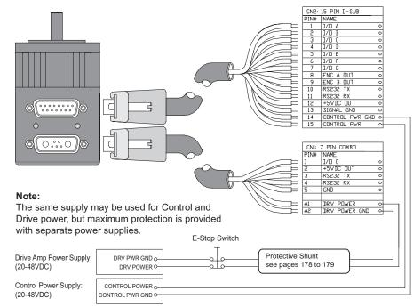
Note: All IP sealed SmartMotors are designed to always have seperate drive and control power. As a result, no DE designation is available for IP sealed SmartMotors. Control power on IP sealed SmartMorors is rated for 24VDC, maximum of 32VDC.
