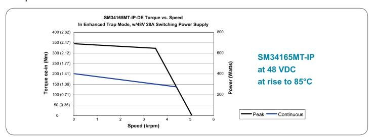
All torque curves were derived under dynamometer testing at an ambient temperature of 25°C with a heat rise of level shown for continuous curves.
