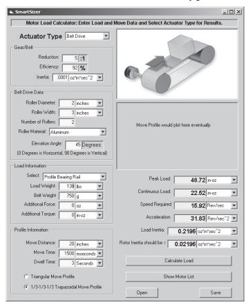
In one simple, single page format, the tool allows the user to fill in values to calculate load torque imposed on a given motor. All input data has a drop down unit selection, allowing you to easily mix and match standard and metric units together.
